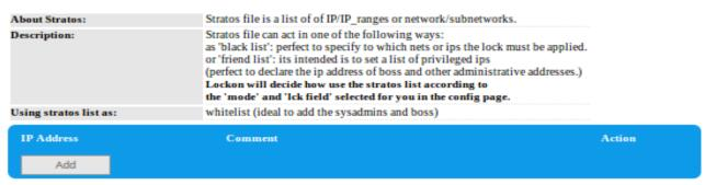
Here, you can add IPs, Networks, Subnetworks depending in the Operation Mode and Lck Field that you set in the main configuration page. You will see a "little tip" of how this list will be used for lockon in front of the "using stratos list as" form.
